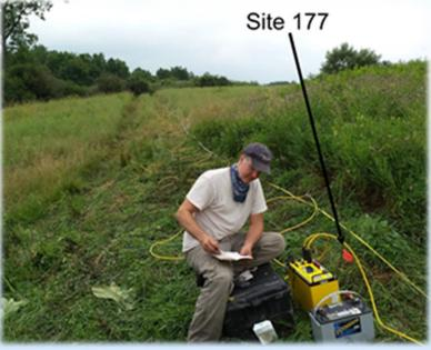
Resistivity Survey in remediated surface-mined area
